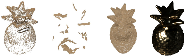
Figure 13: Geometric reconstruction on a challenging object with complex geometry and appearance. From the left to right are our result, the result from a structured-lighting-based 3D scanner [29], single-view photometric stereo [13], and a photograph.
