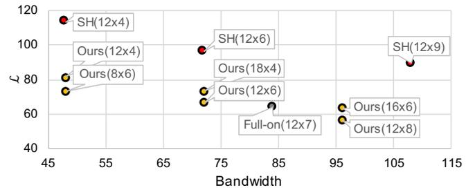
Fig. 9: Comparisons of prediction qualities of networks with different parameters. Parameters  $\#v$  and  $\#l$  are indicated in parentheses as  $(\#v \times \#l)$ . We also add one full-on pattern per-view to our learned patterns ( $12 \times 6$ ) for comparison. The network loss  $\mathcal{L}$  is computed on the validation dataset, according to Eq. 10.
