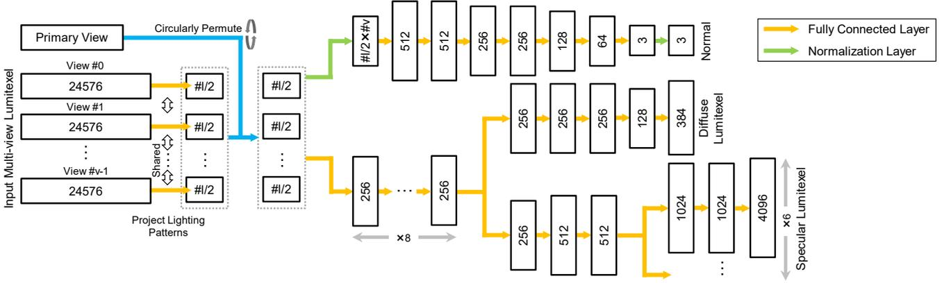
Fig. 7: The architecture of our neural network. The physical multi-view lumitexel of a point  $p$  is transformed into a small number of measurements by a set of lighting patterns shared across all views, implemented as a single fully connected layer. The per-view measurements are circularly permuted according to the primary view. Then they are aggregated to compute a normal, a gray-scale diffuse and specular lumitexel at the primary view as output.
