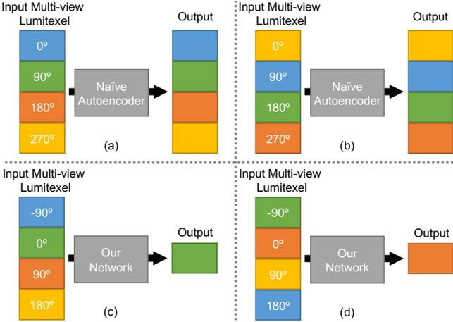
Fig. 4: The structural benefit of our network. The rotational equivariance of input/output must be learned via training data in a naïve autoencoder (a & b). Absolute rotation angles are used here. Our network outputs the lumitexel at one view at a time, assuming only fixed, relative rotation angles with the input views (c & d). This structure explicitly enforces the rotational equivariance. No re-training is needed, if all input views are rotated by a multiple of  $90^\circ$  in this case.
