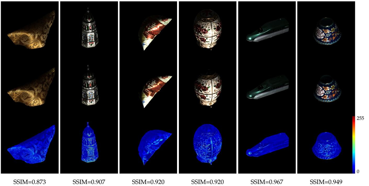
Fig. 15: Validation results. The top row shows photographs of physical objects, the second row are the rendered images of the reconstruction results with our network ( $\#v=12, \#l=6$ ), and the last row shows color-coded differences. The quantitative errors of our results with respect to the photographs are reported at the bottom in SSIM.
