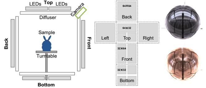
Fig. 2: The lighting layout. From the left to right, a side view of our prototype, the vertical-cross parameterization of all lights with 4,096 LEDs on each face, and the calibration sphere under physically projected *uffizi/stpeters* environment maps.
