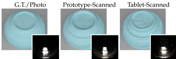
Fig. 9: Comparison of reconstructions of the same object using our prototype and tablet. The main image shows the shape, while the inset is the rendered appearance with novel view and lighting.
