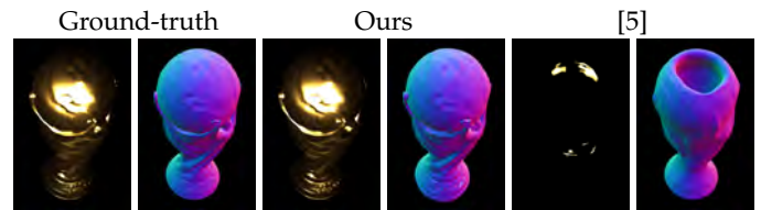
Fig. 10: Comparison between our reconstruction and [5]. For each pair of images, the left one is the appearance rendering, and the right a normal map from the corresponding geometry.
