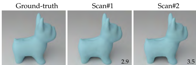
Fig. 15: Repeatability experiment on our geometric reconstruction from 2 scans by 2 different students. Quantitative errors in Chamfer distance are reported in the bottom right corner.
