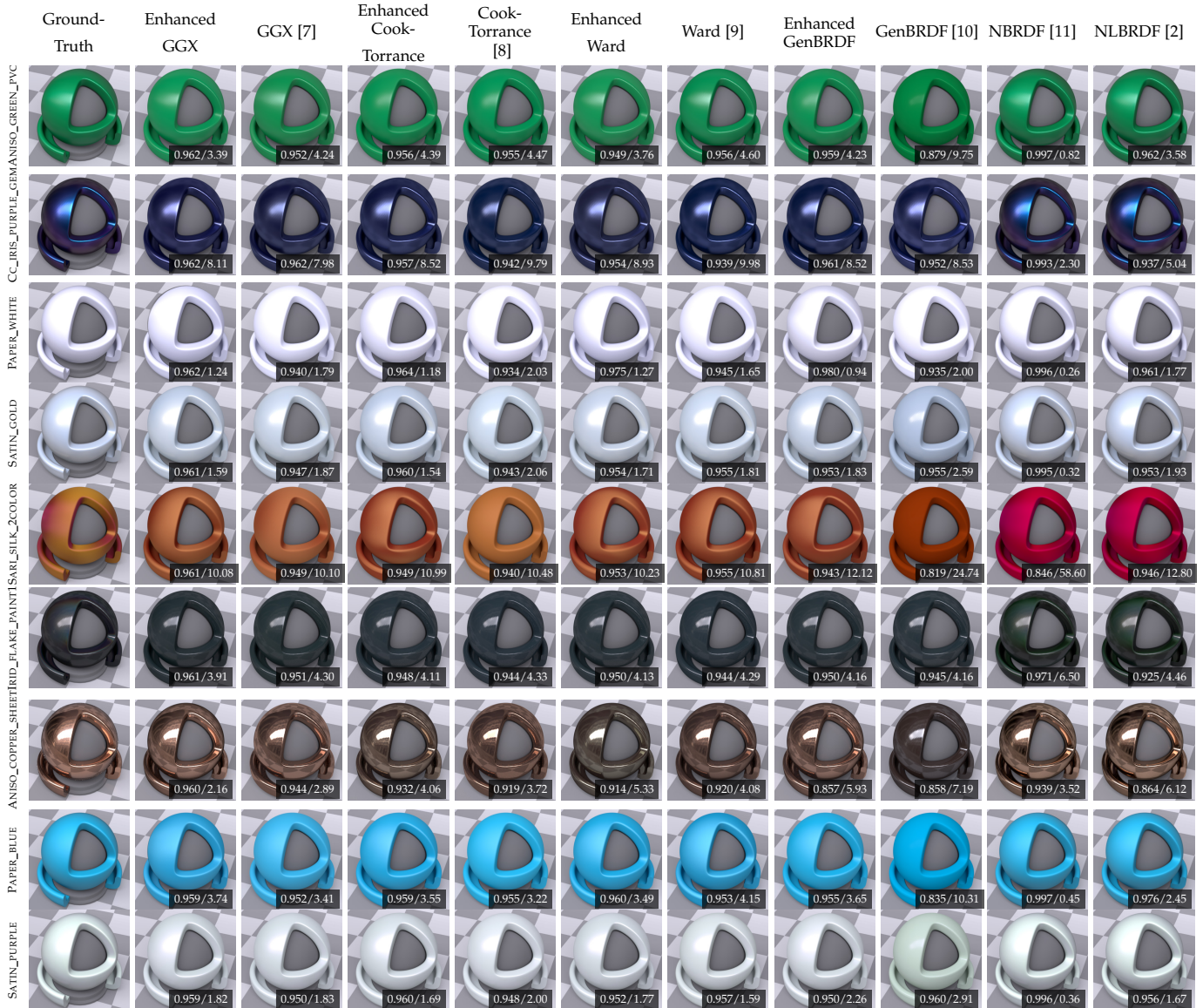
Fig. 3: ( Continued. ) Neural enhancement of several analytical BRDF models on materials from EPFL dataset [5]. From the first column to last, the ground-truths, the results of enhanced/original Cook-Torrance BRDF model with GGX distribution, enhanced/original Cook-Torrance model, enhanced/original Ward model, enhanced/original FULL model in GenBRDF, NBRDF [11], and NLBRDF [2]. Quantitative errors in SSIM and \Delta E_{ITP} ( \times 10^3 ) are reported in the bottom-left of each related image.
