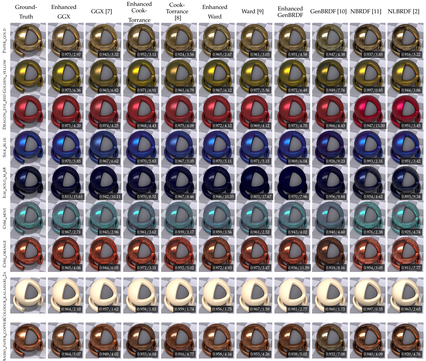
Fig. 3: ( Continued. ) Neural enhancement of several analytical BRDF models on materials from EPFL dataset [5]. From the first column to last, the ground-truths, the results of enhanced/original Cook-Torrance BRDF model with GGX distribution, enhanced/original Cook-Torrance model, enhanced/original Ward model, enhanced/original FULL model in GenBRDF, NBRDF [11], and NLBRDF [2]. Quantitative errors in SSIM and \Delta E_{ITP} ( \times 10^3 ) are reported in the bottom-left of each related image.
