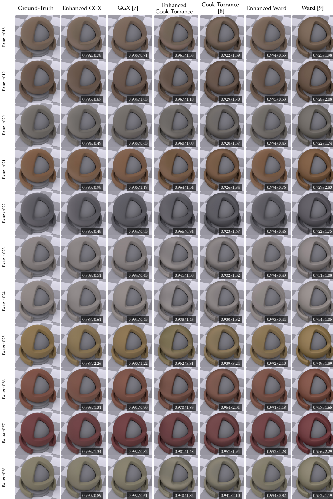
Fig. 4: (Continued.) Neural enhancement of several analytical BRDF models on materials from UTIA dataset [6]. From the first column to last, the ground-truths, the results of enhanced/original Cook-Torrance BRDF model with GGX distribution, enhanced/original Cook-Torrance model, and enhanced/original Ward model. Quantitative errors in SSIM and \Delta E_{ITP} ( \times 10^3 ) are reported in the bottom-left of each related image.
