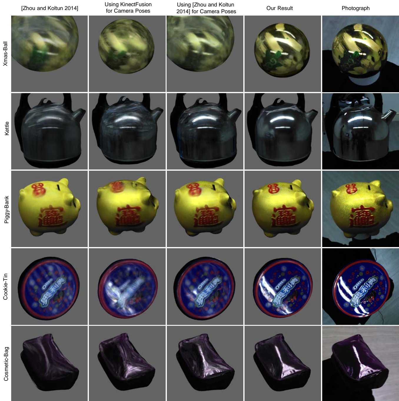
Fig. 13. Comparisons of results using various methods. From the left column to the right: a color-textured model reconstructed by [3], using our method with camera poses obtained from KinectFusion, using our method with camera poses computed by [3], our result and the corresponding photograph (not used in material/lighting/normal optimization).
