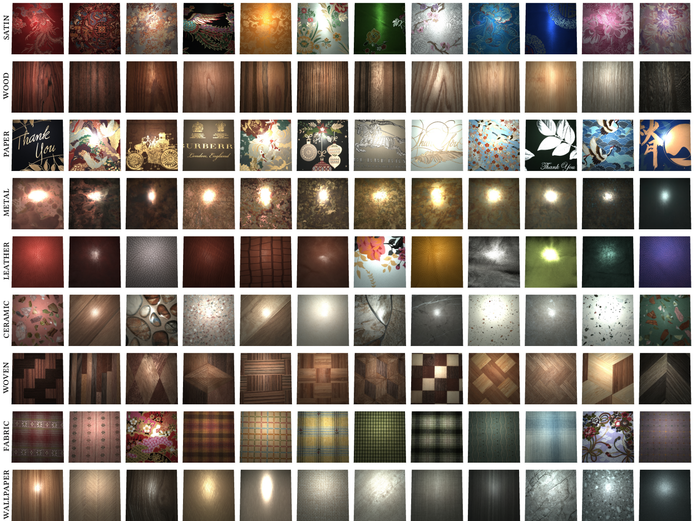
Fig. 1. Rendering results of 108 (out of 1,000) high-quality SVBRDFs captured and reconstructed with our novel integrated system. Each row represents one category in our database. Please refer to the accompanying video for animated sequences.
