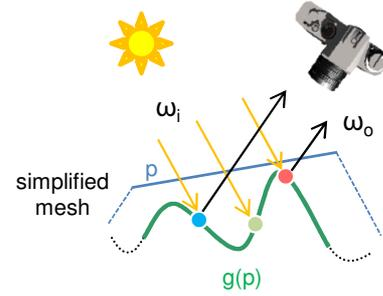
**Figure 5:** Filtered reflectance reconstruction from characteristic points.
