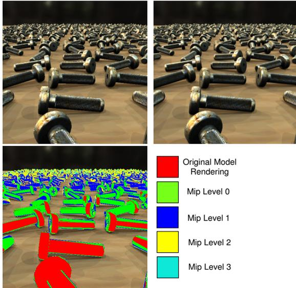
**Figure 9:** An example that shows switching from full model to various levels of CPM representation. Top left: the image rendered with CPMs. Top right: the ground truth rendering of the original model. Bottom: the mip levels color coded.
